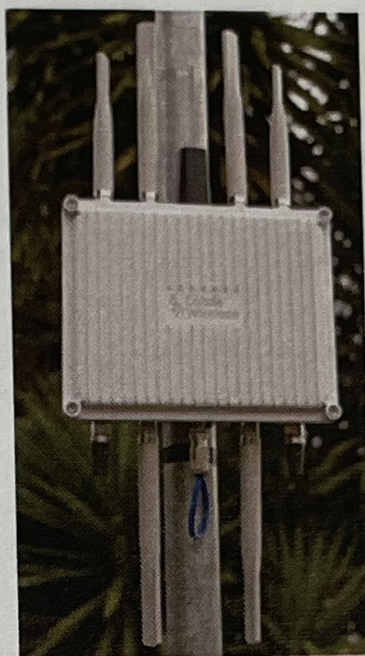
RSU attached to Vertical pole.
