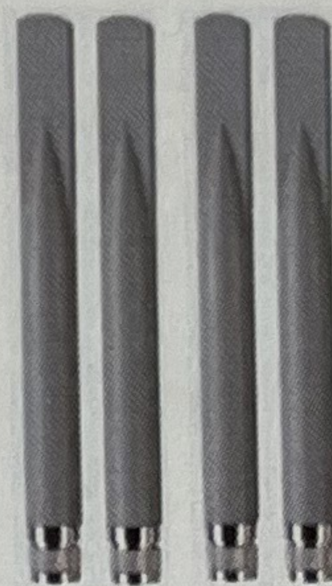
4x 5.9GHz Antennas 2 for DSRC, 2 for C-V2X
